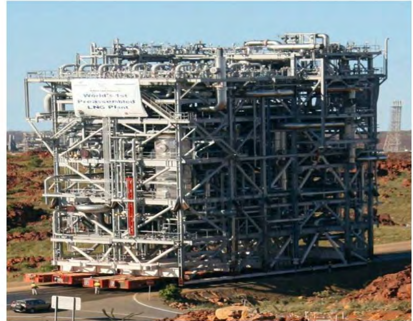
Woodside LNG Train V Expansion Project Module (18,000 tons module weight)
